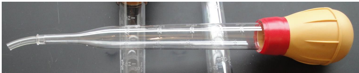
Figure 5. Turkey baster with electrical tape wrap (red) and segment of 1/8” soft aquarium tubing.
