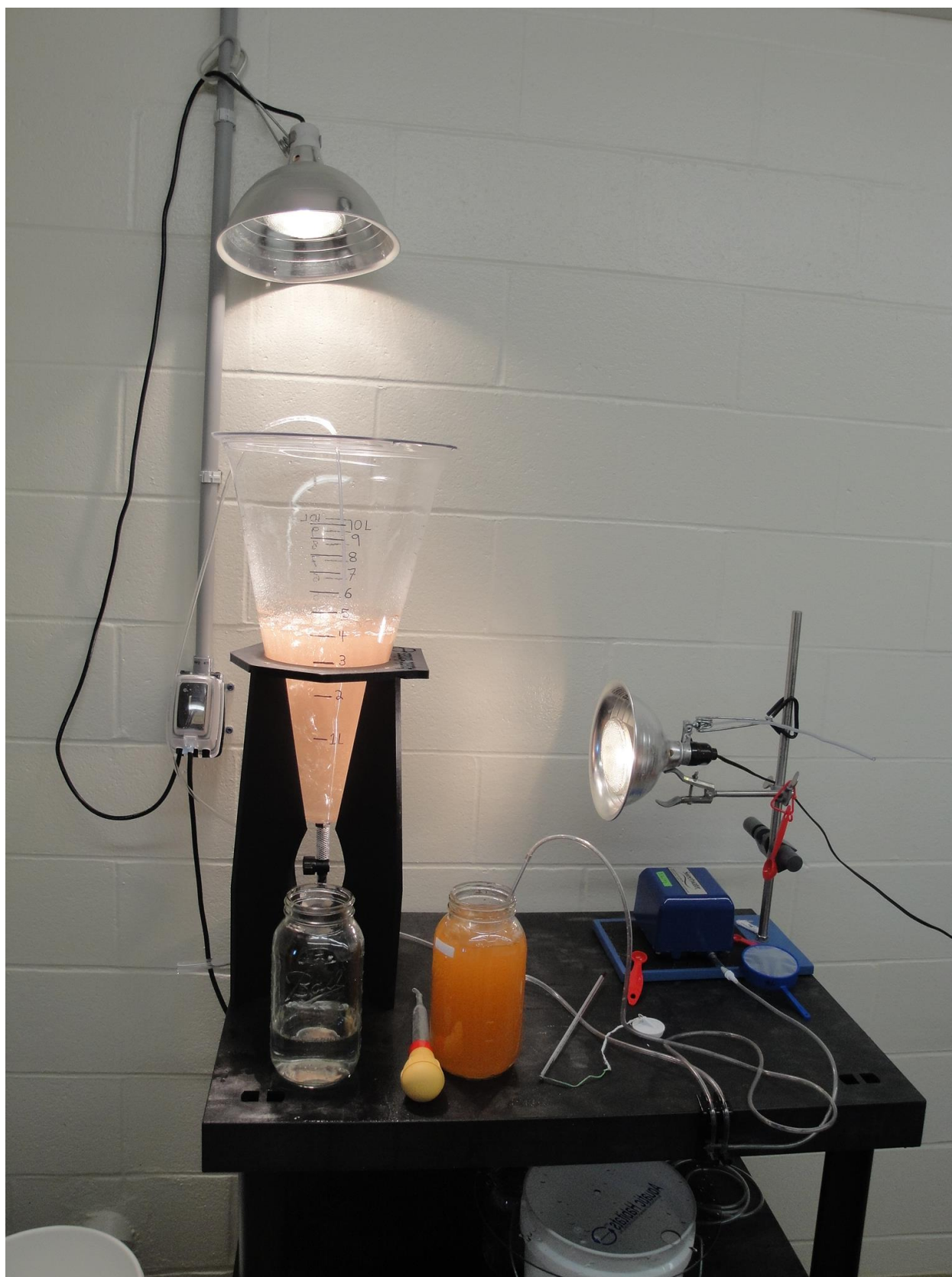
Figure 1. The Aquatic Habitats brine shrimp hatchery. The many additional components include lights, ring stand, air pump, tubing and valves, buckets, ½ gallon jars for seawater and nauplii suspension, measuring spoons for cysts, collecting sieve, baster for dispensing, and thermometer.
