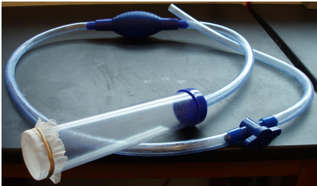
Figure 10. Lee's Ultra Gravel Vac ® fitted with a 2-mm nylon mesh cover to prevent the inadvertent suction of stickleback larvae. The cover impedes removal of large debris and should be removed when fish are large enough to avoid the vacuum.
