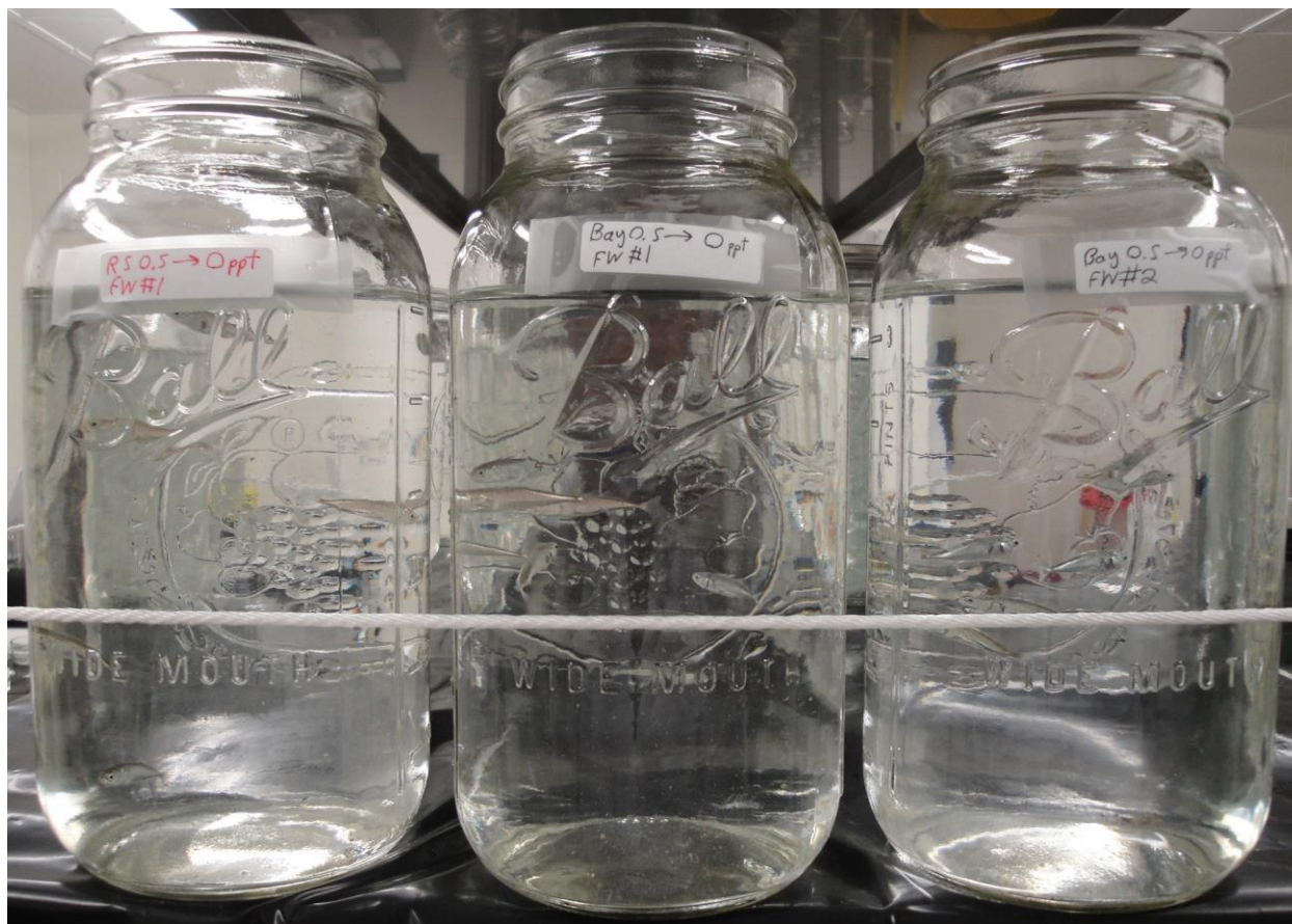
Figure 7. Wide-mouth glass mason jars are the most widely used item in stickleback husbandry. Pint jars are used to prepare food, quart jars house larvae, while the half-gallon (pictured) is the best size for salinity challenge experiments on juveniles.
