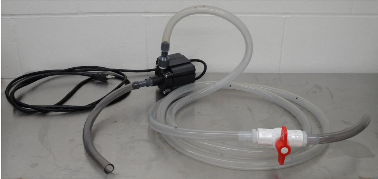
Figure 8. One of two 350 gph submersible pumps attached to ½” barbed fittings and vinyl tubing. The shorter intake hose sucks water from the bottom of the barrel, which will then exit through the long hose, regulated by a ball valve.
